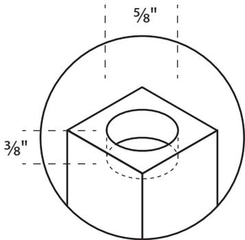
Use a depth stop on the drill press to keep the holes consistent
